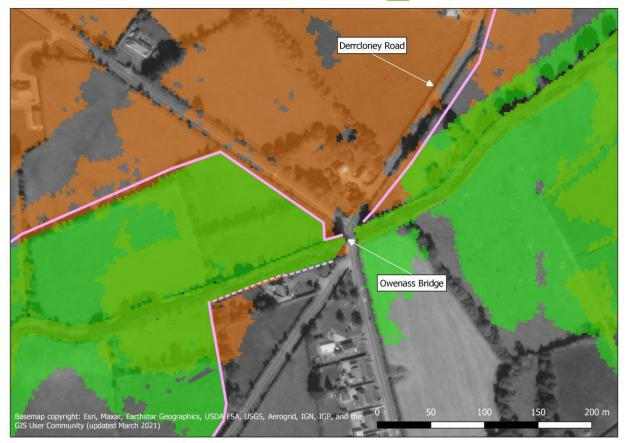
Description: In Option 2A, the floodplain embankment results in increased flooding to the east of the Owenass. As a result properties around Owenass bridge that were previously not flooded are impacted in Option 2A. Defences in the form of walls and embankments will be required around these properties (flood level around defences approximately 0.90m or just under 3').
