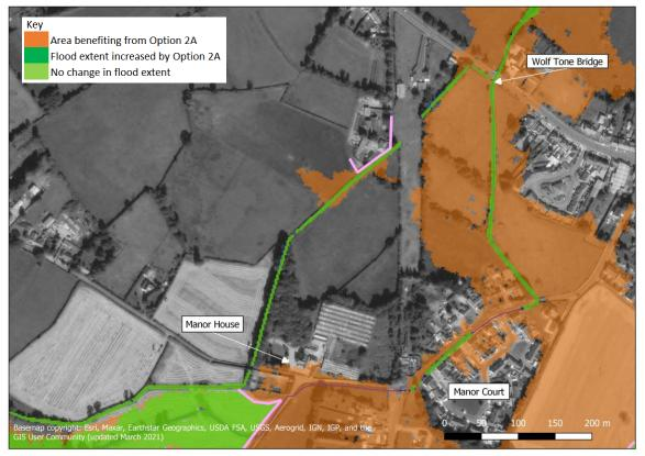
**Description:** Under Option 2A, there is an increase in flows down the Garroon. As the culvert below the old railway line is under capacity, water backs up and creates a flood risk to property to the north. This may be managed
