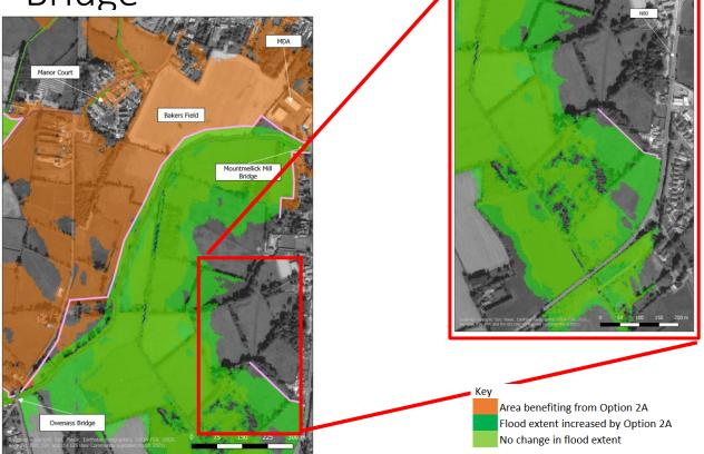
**Description:** The defence line follows the left (westerly) bank of the Owenass at an offset of 30-40m. This protects the floodplain from flooding when compared with the current scenario. However, flooding on the eastern bank of the Owenass increases in extent and depth and as a result a length of embankment is needed to protect the garden centre.
