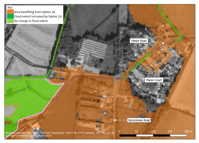
**Description**: In Option 2A, the combination of the main Owenass embankment and the Pound embankment and throttle means that no additional defences are needed along the Manor Road channel as the flow is low enough that the system can pass it though.
