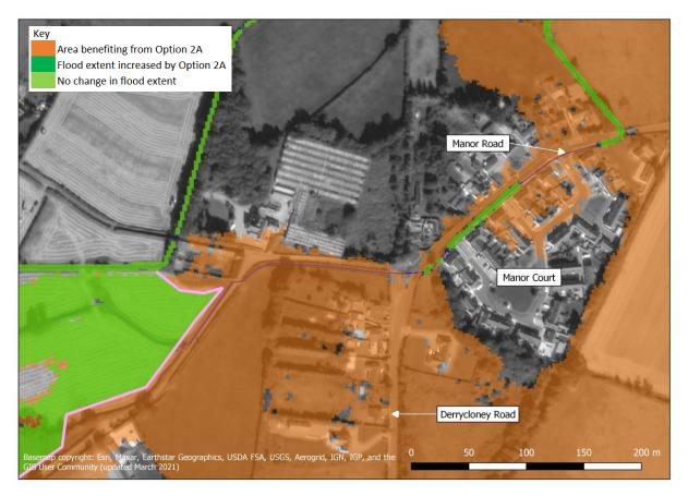
**Description:** The main Owenass embankment blocks cross floodplain flow to the Pound. The Pound is better able to manage the reduced flows. In Option 2A an embankment to west of Sandy Lane, in the vicinity of the old mill pond provides a flood storage area. A throttle below the embankment further limits flows down the Pound. As a result of the reduction in flows from the Owenass, flood depths at this location decrease by approximately 30cm (12") compared to the current scenario.
