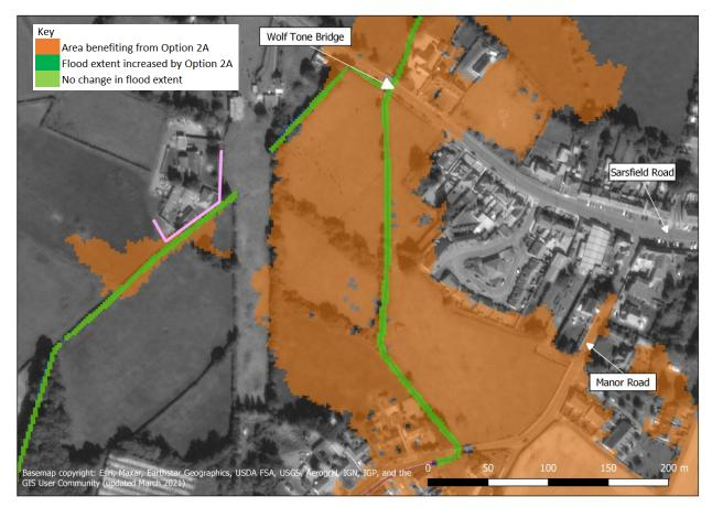
**Description**: In Option 2A, the combination of the main Owenass embankment and the Pound embankment and throttle means there is no flooding modelled in this area. Therefore there is no need for defences along Wolfe Tone bridge or around the property boundaries.
