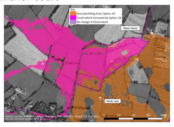
**Description:** The main Owenass embankment blocks cross floodplain flow to the Pound. The Pound is better able to manage the reduced flows. In Option 2B an embankment to west of Sandy Lane, in the vicinity of the old mill pond provides a flood storage area. A throttle below the embankment further limits flows down the Pound. As a result of the reduction in flows from the Owenass, flood depths at this location decrease by just under 30cm (12") compared to the current scenario.
