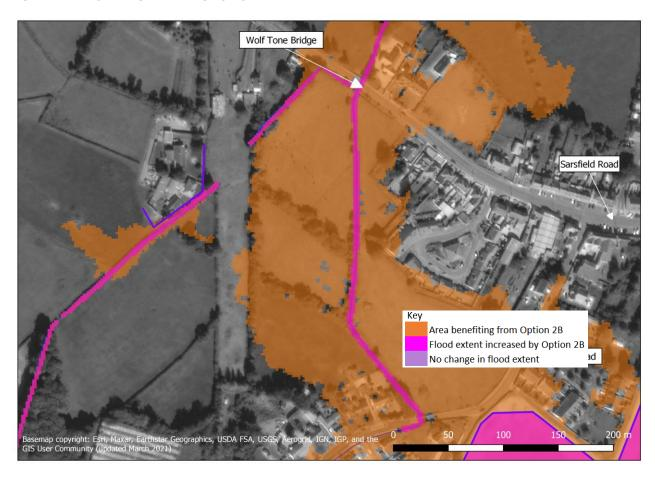
**Description**: In Option 2B, the combination of the main Owenass embankment and the Pound embankment and throttle means there is no flooding modelled in this area. Therefore there is no need for defences along Wolfe Tone bridge or around the property boundaries.
