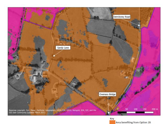
**Description:** As with Option 2A, the embankment along the Owenass prevents flooding of the properties in the floodplain upstream of Mountmellick town. The embankment blocks the cross flow removing the flood risk to these upstream properties and land.
