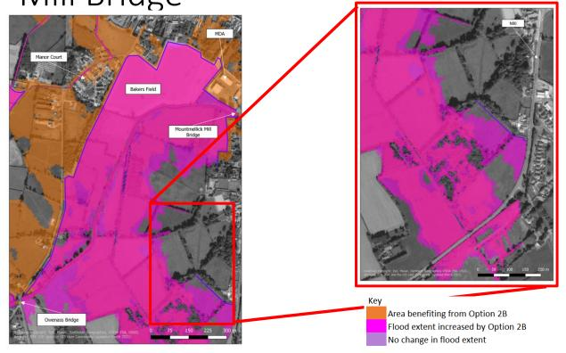
**Description:** The defence line is tight to the line of urban development and follows the northern boundary of the Baker's field and perimeter of the MDA lands. It then follows the Derrycloney Road to the south and continues past the Owenass Bridge. The west bank of the Owenass is flooded in the undefended scenario and continues to be flooded when Option 2B is in place as
