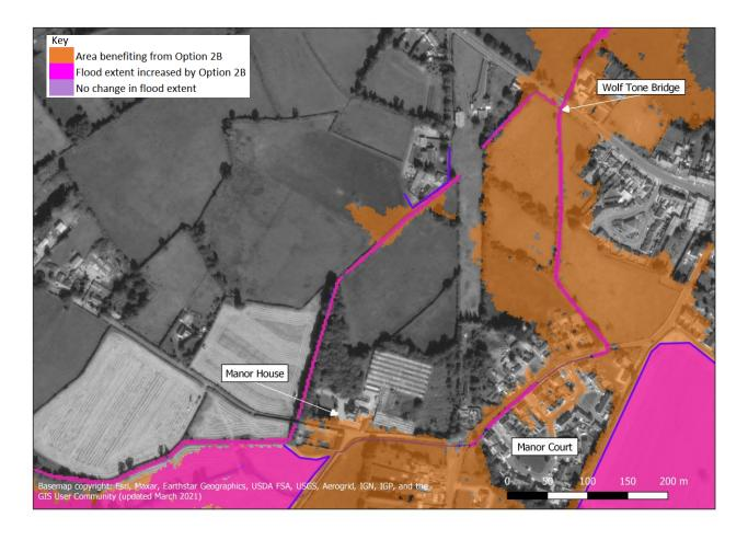
**Description:** As with Option 2A, under Option 2B there is an increase in flows down the Garroon. As the culvert below the old railway line is under capacity, water backs up and creates a flood risk to property to the north. This may be managed
