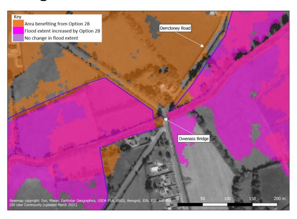
**Description:** As with Option 2A, in Option 2B, the floodplain embankment results in increased flooding to the east of the Owenass. As a result properties around Owenass bridge that were previously not flooded are impacted in Option 2B. Defences in the form of walls and embankments will be required around these properties (flood level around defences approximately 0.90m or just under 3').
