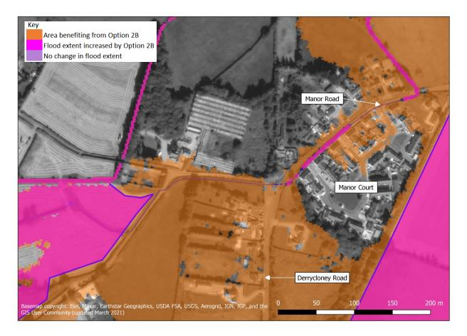
**Description**: In Option 2B, the combination of the main Owenass embankment and the Pound embankment and throttle means that no additional defences are needed along the Manor Road channel as the flow is low enough that the system can pass it though.
